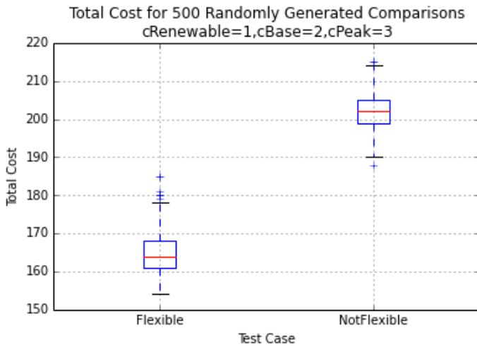
Fig. 6. Monte Carlo analysis of cost for 500 randomly generated simulations with ‘smart’ and ‘dumb’ appliances
